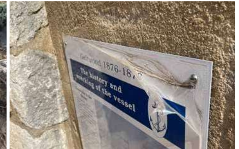
Geltwood interpretive signage - wrong materials, poorly fabricated and de-laminating
