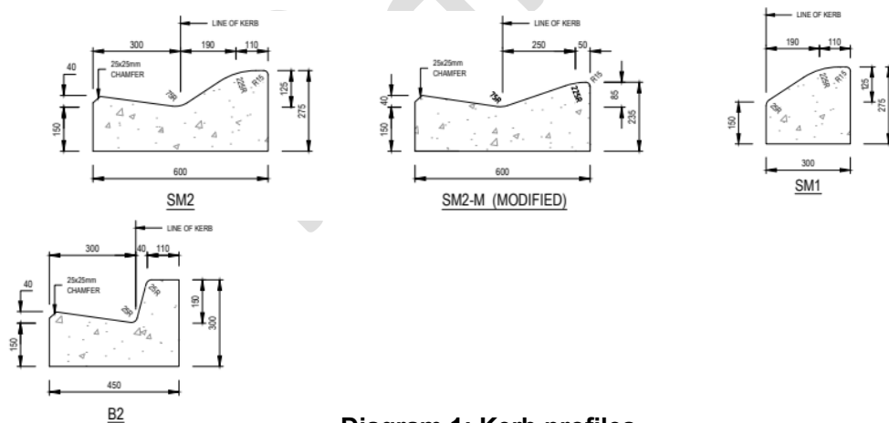
Diagram 1: Kerb profiles
