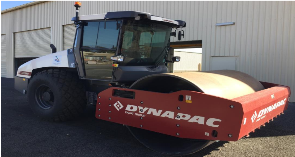
New Vibrating compactor roller
