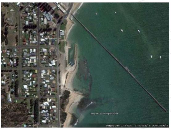
Figure 4.1 – Aerial view of the current boat ramp and marina basin arrangement. The central sand bar can be seen in the middle of the basin (Source: Google Earth, March 2016)
