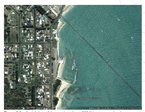
Figure 3.6 – Aerial view of the previous (post 2004) boat ramp showing waves transforming around the geotextile bag breakwater. (Source: Google Earth, October 2012)
