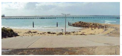
Photograph 3.10 – View to North-East of the previous Boat Ramp during winter months showing the large build-up of sand on the beach. Note that the ramp is entirely ineffective and floating pontoons have been removed. (Source: Author, August 2010)
