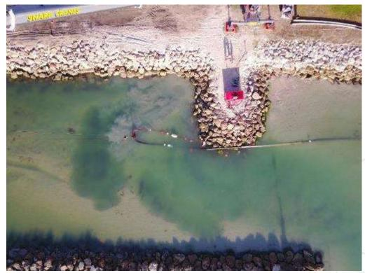
Photograph 5.4 – Drone view of dredge trial underway (Source: Maritime Constructions, March 2017)
