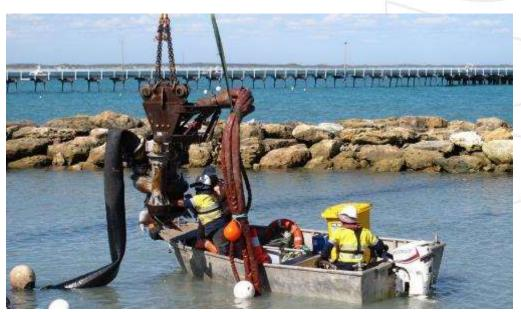
Photograph 5.11 – Dragflow pump being cleared of seaweed from the intake screen (Source: Author, March 2017)
